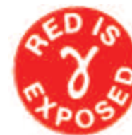
60 Co irradiation exposed sticker as sterility indicator
