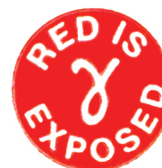
60 Co irradiation exposed sticker as sterility indicator
