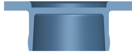
Indented qPCR Cap, the optical area is recessed into the optical cap surface to prevent "touching" the optical area.
