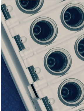
Detail of an 8 Tube-Strip Mat 0.1 ml LP (ultra clear), “clicked in” into a white FD Full Skirted grid (B1679FD or B679FD).
